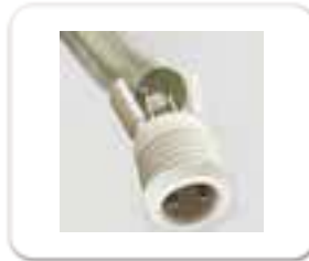
Align the self-piercing pins with the conductors in the rope light. Once the pins are aligned push the pins into the rope light, keeping the pins aligned with the conductors. Rounded pins mate with plug.
