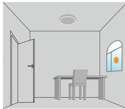
Lights off when ambient light level is higher than preset lux value.
