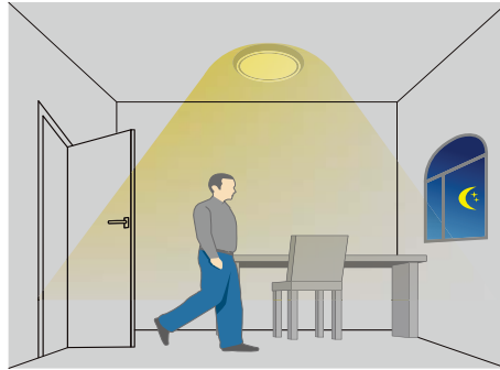
With insufficient ambient brightness, light dims to 100% when motion detected.
