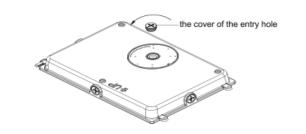
4. Put the input line in the embedded box passes through the waterproof pad and then passed through the lamp base.
