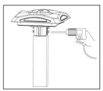
2) Lock the screws on both sides of the lamp, fix the lamp to the pole.
