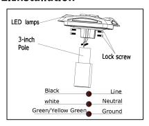
1) Connect the AC wire of the lamp as shown in the picture, then insert the lamp into the 3-lnch pole.
