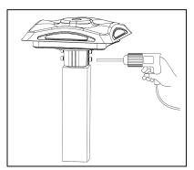
2) Lock the screws on both sides of the lamp, fix the lamp to the pole.
