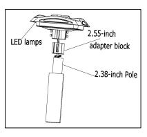
3) When the light pole is 2.38 inches, a 2.5 inch adapter shall be installed on the fixture.
