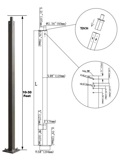
Series Straight Square Steel poles are built from high strength steel tube and are available side drilled for arm mounted area lighting luminaires or with tenon mounts for flood and post top luminaires. Typical area lighting applications include retail centers, industrial parks, schools and universities, public transit and airports, office buildings and medical facilities. Mounting heights of 10 to 30 feet can be used based on selected luminaire application.
