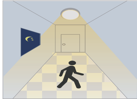
With insufficient daylight, when motion detected, light ON.
