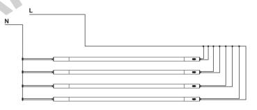
Step 2. For non-shunted holders, wire the holders and lamps according to the diagram.
