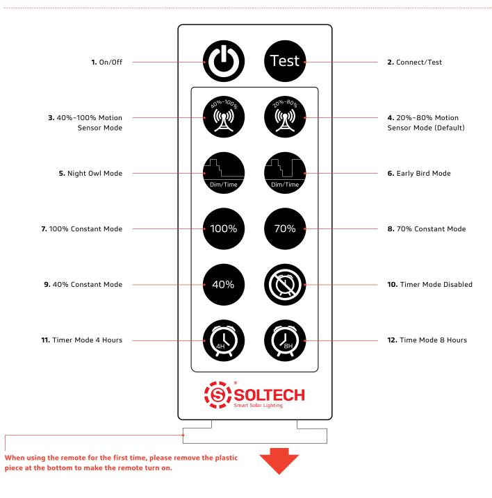
The range of the remote control to the indicator is 16ft (Day time) to 33ft (Night time). Because the sunlight will impact the signal of the remote control, we suggest our users to setup the mode before they install the light.
