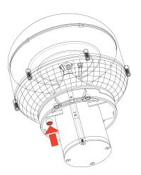
When installing the wall mount base, please put Part A and Part B into the surface holes first then install the wall mount base on top.
