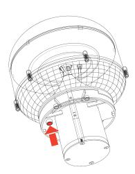
When installing the wall mount base, please put Part A and Part B into the surface holes first then install the wall mount base on top.
