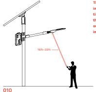
The range of the remote control to the indicator is 16ft (Day time) to 33ft (Night time). Because the sunlight will impact the signal of the remote control, we suggest our users to setup the mode before they install the light.
