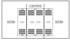
**3.** Break **bracket** into three pieces. (Side bracket for RXL-4 and 8. Centre bracket for RXL-8 only)
