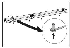
**6.** Fasten **safety lanyards** to fixture by using provided **tek screws** and washers.
