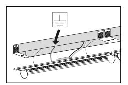
**8.** Connect ground cable to incoming ground lead from conduit.
