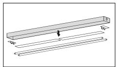
**2.** Remove original lamps, ballast cover, and sockets.
