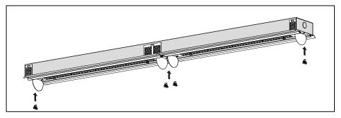
**11.** Secure the **LED gear tray** to the **brackets** by inserting the **quarter turn fasteners** into the holes and turning 90 degrees. Use pliers if needed.
