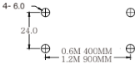
drill hole size of ceiling installation
