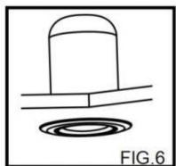
If the installed housing does not have TORSION SPRING SLOTS or C-CLIPS (FIG. 5), then remove the SCREWS securing the TORSION SPRINGS to the HEATSINK. Attach the FRICTION BLADES (included) to the same location using the SCREWS that were previously removed. (FIG. 6)
