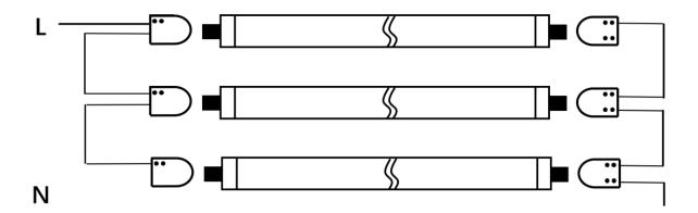
• Step 3: Affix the field applied label to the light fixture and install the tube. The tube is double ended wiring connection.
