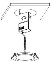
8. Lifting both retention tabs upward, push the fixture into the hole until trim sits flush with ceiling.
