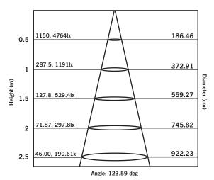
Note: The curves indicate the illuminated area and the average illumination when the luminaire is at different distances.
