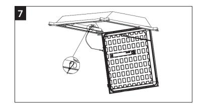
8. Close the retrofit kit door into the fixture and rotate the clips to secure the door closed.
