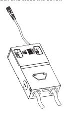
Insert driver box into ceiling in accordance with local/ national codes and connect the male and female connectors. Screw threaded nut over connectors to secure.
