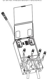
**6.** Place all wiring and connections back into the box and close the cover.
