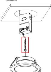
8. Lifting both retention tabs upward, push the fixture into the hole until trim sits flush with ceiling.
