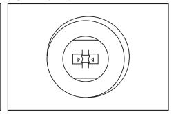
**4.** Access sign raceway/wiring box, and cut all ballast input and output wires as shown. Do not remove ballast if removal leaves an opening in the raceway.
