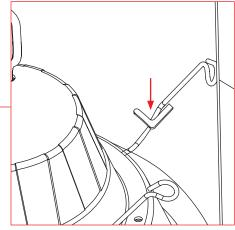
**8.** Carefully place wires into housing, then push the LED trim into the housing until trim is flush with ceiling.
