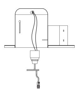
**5.** Select desired CCT using adjustment switch on driver box (see *Color Select* (*CCT*) *Adjustment* on page 3).
