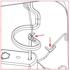
6. Carefully place wires into fixture, then push the LED trim into the housing until trim is flush with ceiling.
