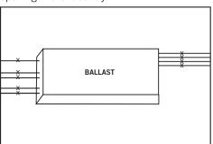
**5.** From mains, connect input (L) line to all wires coming from sockets on one side of sign and (N) neutral to all wires coming from the sockets on opposite end of the sign.
