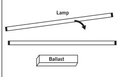
**3.** Inspect existing sockets to ensure they are in good shape, replace if needed.
