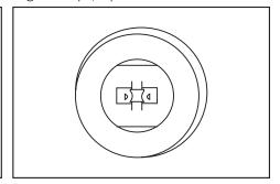
**4.** Access sign raceway/wiring box, and cut all ballast input and output wires as shown. Do not remove ballast if removal leaves an opening in the raceway.
