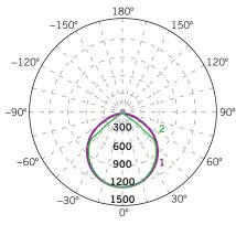
Average Beam Angle =  $160.0^{\circ}$ Located at Horizontal Angle = 0Vertical Angle = 0
