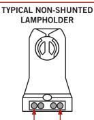
Connect wires directly to these terminals
