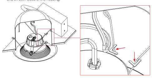
8. Carefully place wires into the fixture, then push the LED trim into the housing until trim is flush with ceiling.
