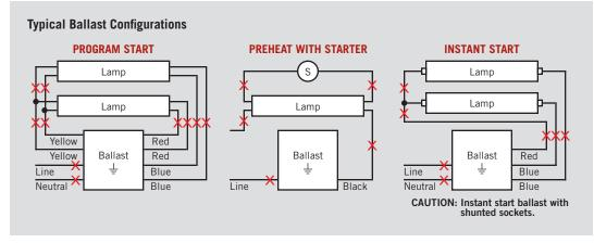
Single-ended wiring without dimming: Re-wire fixture as shown below.
