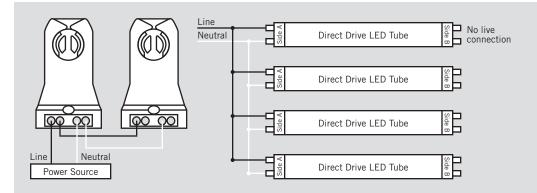
Single-ended wiring with dimming: Re-wire fixture as shown below.
