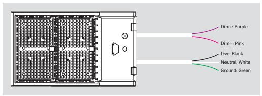
• This fixture comes pre-wired with a 7-pin twist-lock receptacle with shorting cap.
