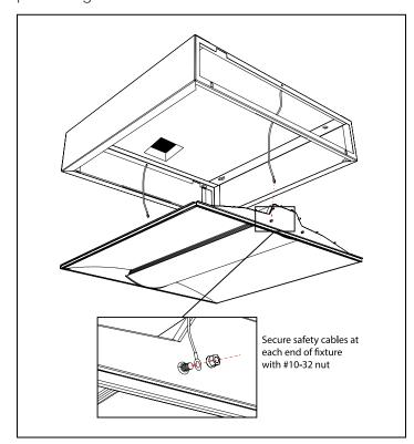
2. Secure end plate to one side of surface mount frame by securing clips to frame edge and rotating slots into studs on frame. Secure using two #10-32 nuts.
