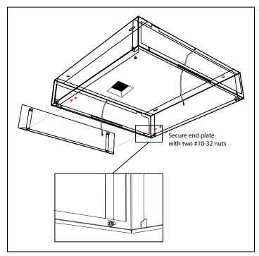
**4.** Make all electrical connections according to local code and make sure safety cables are secure. Angle the fixture into the bottom flange of the surface mount kit between locating tabs on all four corners. If the fixture is not resting properly on the bottom flange, lift it up and shift it until it rests into place.
