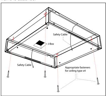
3. Prior to wiring fixture, secure safety cables at each end of the fixture by at tacking to the existing protruding screws and secure with #10-32 nuts.
