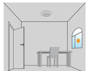
Light off when ambient lux level is higher than preset lux amount.
