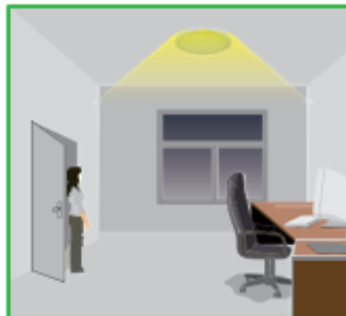
With insufficient natural light, the sensor switches on the light automatically when person enters room.
