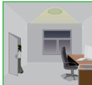
People left, light still dims to 0/10%/30%/50% (options) standby level after the hold time.
