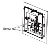
2.Unscrew the cover of the entry hole on the lamp base and remove the cover.
