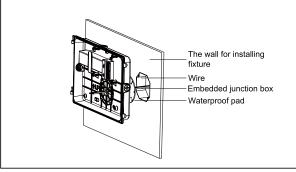
6.Connect the input wire and the dimming wire of the light, then put the connect ed wires into the embedded terminal box.
