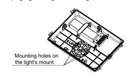
5.Use screw to lock the lamp base on the embedded junction box.
