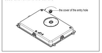
4. Put the input line in the embedded box passes through the waterproof pad and then passed through the lamp base.
