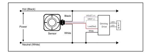
**BRI819-O** wiring with non-dimming ballast or LED driver. **ON/Off Sensor**
