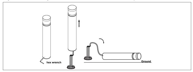
5. Place bollard base plate over anchor bolts and tighten nuts securing the base plate to the foundation. Double check the wires are in good connection after the base installation.
