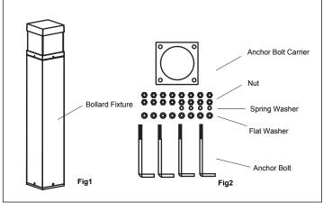
2. Prepare site. Get the anchor bolt carrier assembled as Fig 3 and use it to determine placement of anchor bolts in concrete. Ensure that concrete base is suitable for the bollard load.
