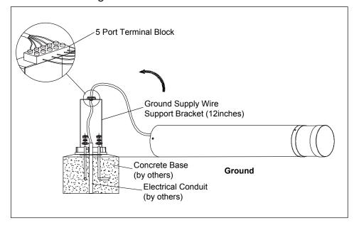
6. Put back the fixture body, and tighten the set screws (x3) with hex wrench.
