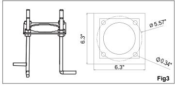
3. Install three anchor bolts into concrete as per attached drawing, having at least 1-1/2~2" protruding from concrete with threads free and clear of debris and dirt.
