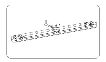
4.Fix the lamp to the ceiling with the plastic sleeve and screws provided.
