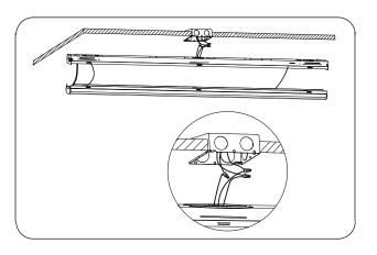
2.Fix the baffle on the lamp.
